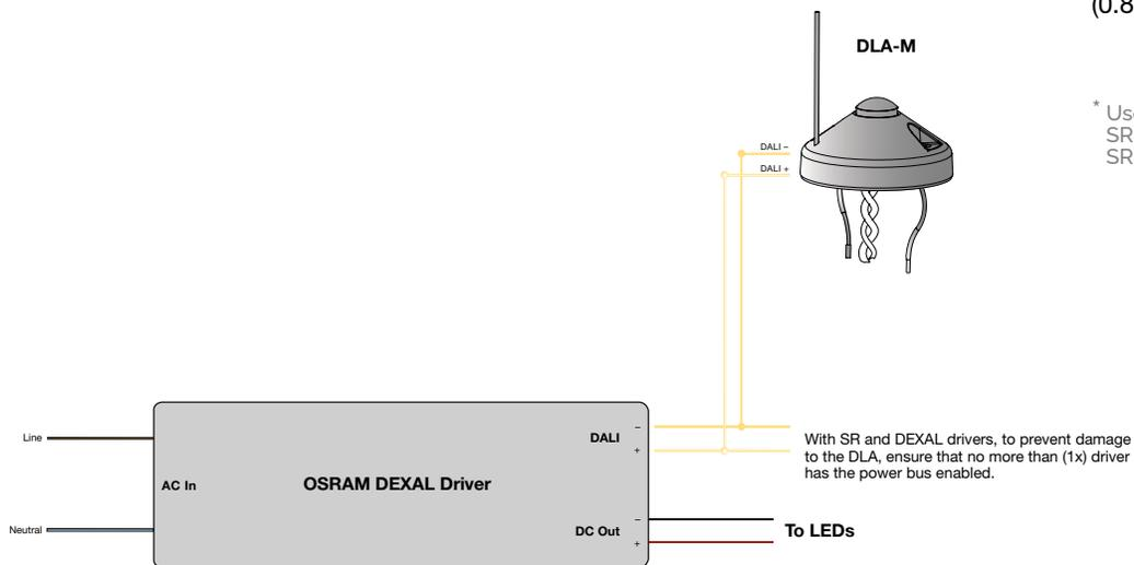
**Note:** Use 18 to 22 AWG (0.82 to 0.33 m<sup>2</sup>) wiring
