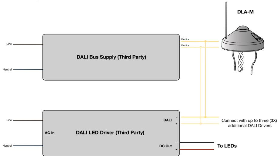
**Note:** Use 18 to 22 AWG (0.82 to 0.33 m<sup>2</sup>) wiring
