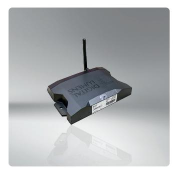
The **DLGW3** Wireless Network Gateway provides simple and secure communication between Siteworx Software Smart Devices and the SiteWorx® Facility Insights Application Suite, enabling data acquisition and providing insights and actions — improving facility efficiency and energy savings.
