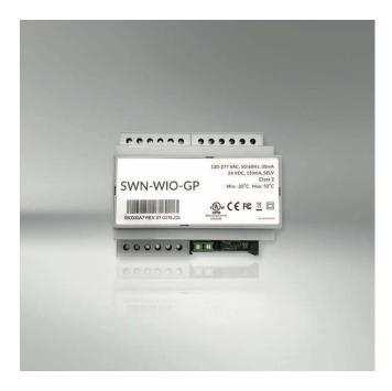
The **SWN-WIO** is a wireless, multi-function, DIN rail-mounted Input/Output module that integrates many sensory devices and load control capabilities with SiteWorx Sense.
