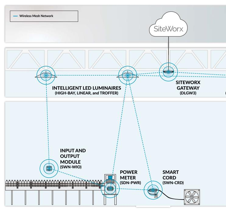
Wireless sensors and meters transmit important facility data such as temperature, humidity, pressure, vibration, flow rate, and power characteristics to SiteWorx using the Wireless Mesh Network.
